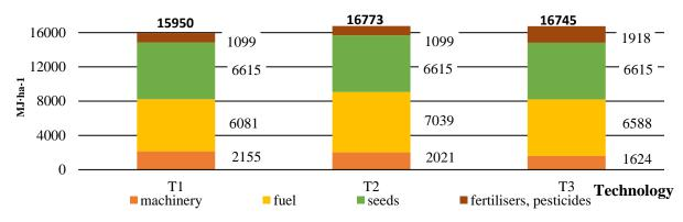
Fig. 2. Technology energy input, calculation by components
